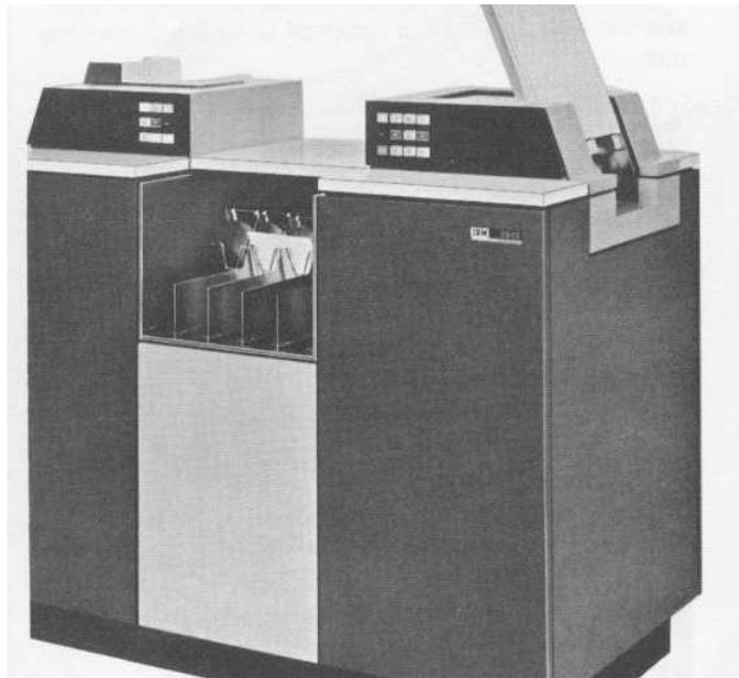
**Figure 6 IBM 2540 Card Reader/Punch**
