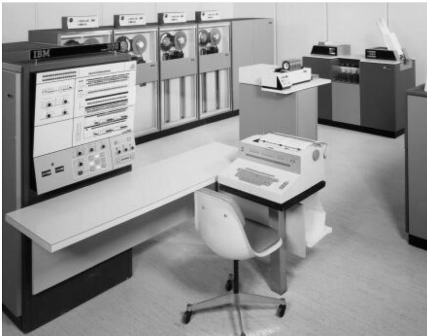
**Figure 3. Computer console is on the far left. The punched card reader is against the back wall on the right. The cables connecting the various devices run beneath the floor.**
