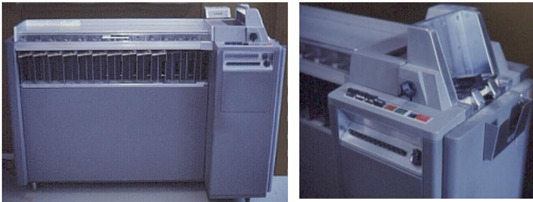
**Figure 8 Punched Card Sorter. The knob in the center of the right photograph is the dial that selects a specific column to be sorted.**
