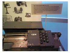
keypunch put round holes in 45 column cards. When IBM switched to 80-column cards with rectangular holes in 1928, many machines were reconfigured to the new standard, including this one."
