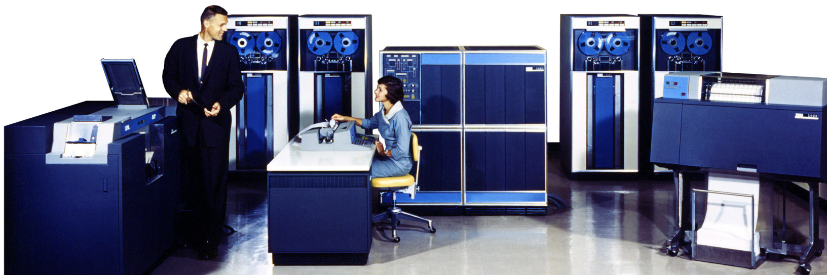
IBM 1401 system. From left to right: 1402 (card reader), 729 (tape drive), 1407 (console), 1401 (CPU), 729 , 1403 (printer)
