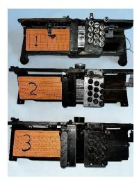
Number 1 is our punch, 2 and 3 are verifiers. At that time the punch was not punching and we had no need for verifiers. Frank wondered if I might fix the punch, and I wondered if a verifier could be converted to a punch. I borrowed all three machines so I could work on them in my home lab. I started by dissembling machine 3. In this report I will skip over a few months of learning and testing.
