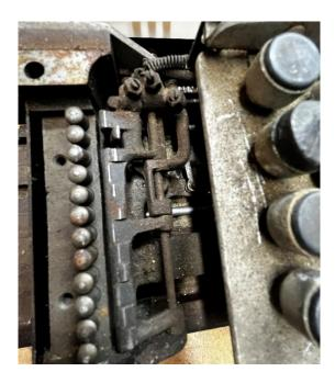
When the device is configured as verifier, one of the parts (skiplever item 35) is ¼" longer and eliminates the interlock completely. This longer part also avoids a tolerance issue in the toggle logic.
