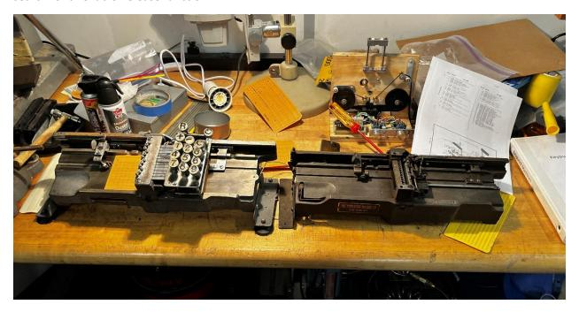
The Release function is implemented by setting a mechanical latch which lifts an escapement pawl holding the carriage. When the pawl is lifted a spring returns the carriage to column 1. The latch and pawl are reset end of travel. At this point the escapement is in it normal state, controlling the movement of the carriage one column with each button press.
