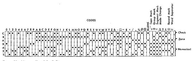
Figure 86. Magnetic Tape 7-Bit Coding
