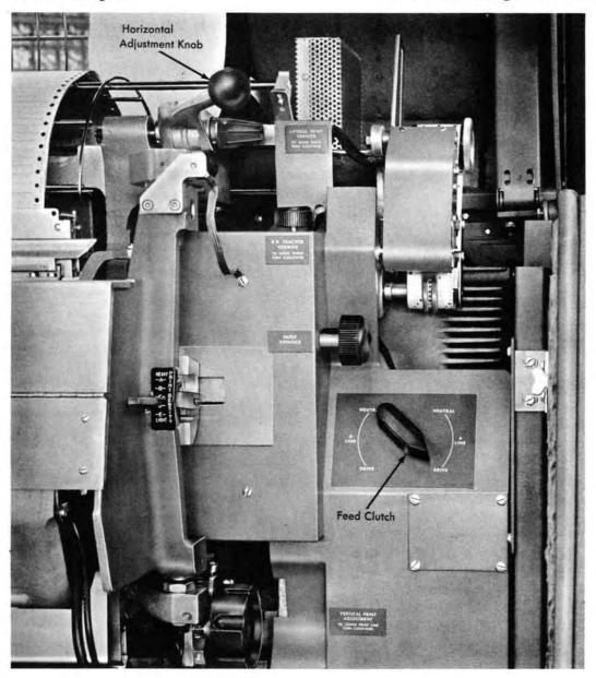
Figure 200. Manual Controls
