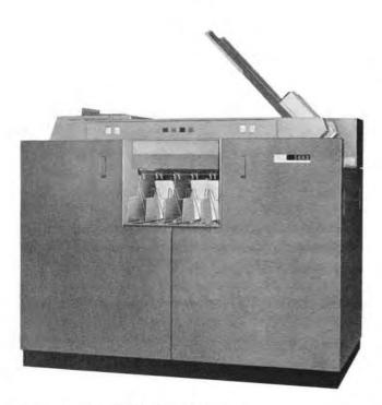
Figure 4. IBM 1402 Card Read-Punch
