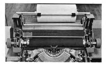
Figure 219. Removing the Platen
