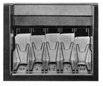
Figure 6. Radial Stackers
