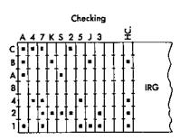
Figure 87. Vertical and Horizontal Check
