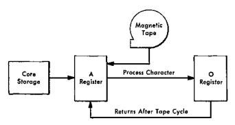
Figure 175. Overlapped Read Magnetic-Tape Operation
