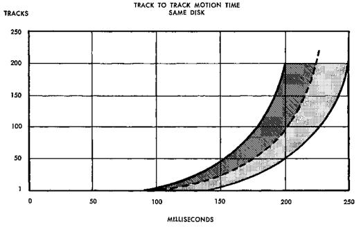
Figure 253. Track-to-Track Motion Time-Same Disk
