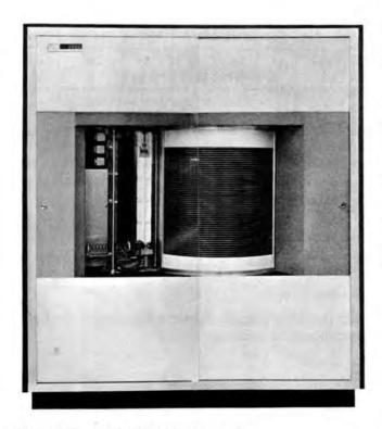
Figure 109. IBM 1405 Disk Storage Unit
