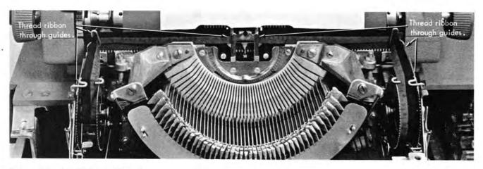
Figure 218. Console Printer Ribbon
