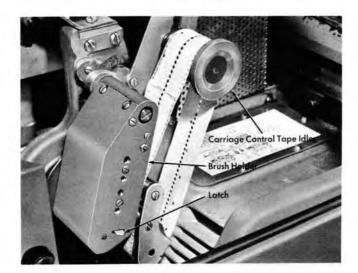
Figure 205. Tape-Contolled Carriage
