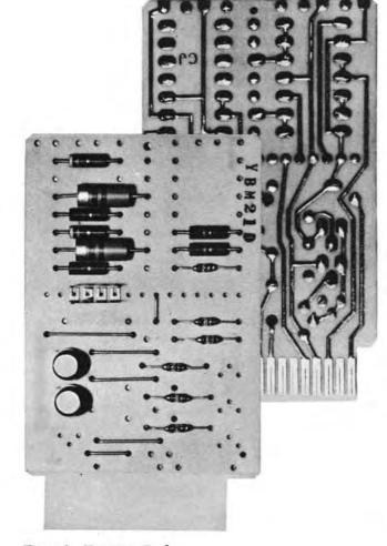
Figure 2. Transistor Cards
