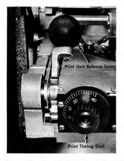
Figure 201. Print-Timing Dial and Print-Unit Release Lever
