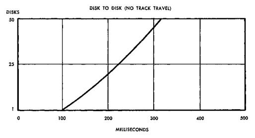
Figure 254. Disk-to-Disk Travel (No Track Travel)
