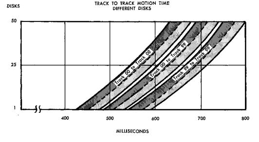
Figure 252. Track-to-Track Motion Time-Different Disk
