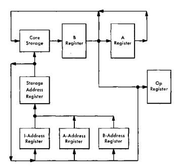
Figure 16. IBM 1401 Processing Unit Registers
