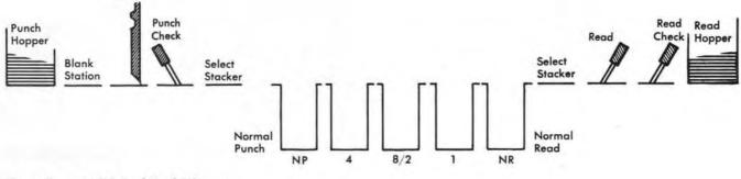
Figure 5. IBM 1402 Card Feed Schematic
