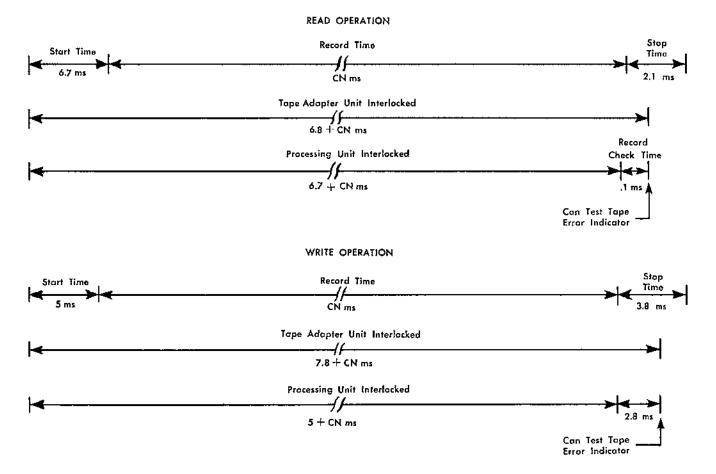
Figure 246. IBM 729, Model IV, Read-Write Tape Timing
