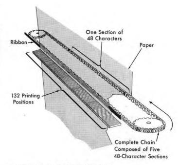
Figure 8. Printing Mechanism Schematic
