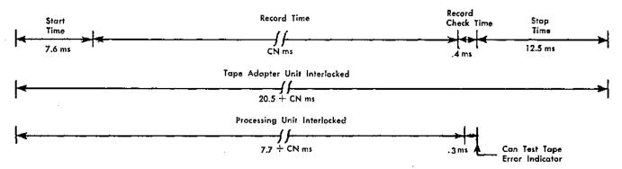
Figure 247. IBM 7330 Read Tape Timing
