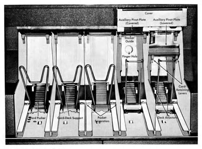
Figure 171. 51-Column Adjustable Stackers
