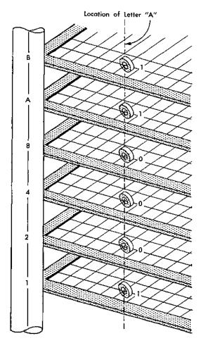
Figure 10. The Letter A Represented in Magnetic Core Storage
