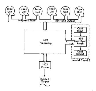
Figure 85. Data Flow Schematic, IBM 1401
