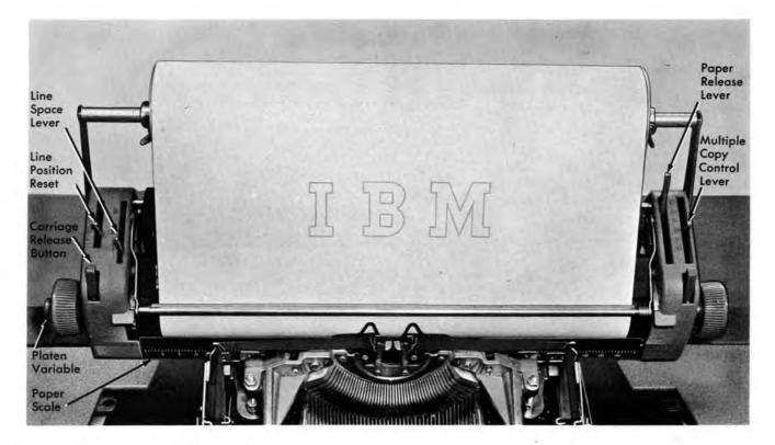
Figure 216. Impression and Carriage Control
