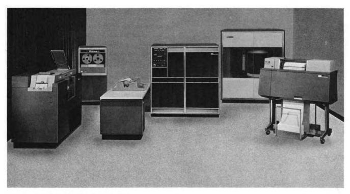
Figure 1. IBM RAMAC 1401 Data Processing System
