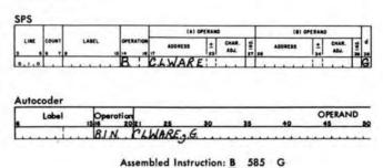
Figure 157. Test and Branch if Indicator On
