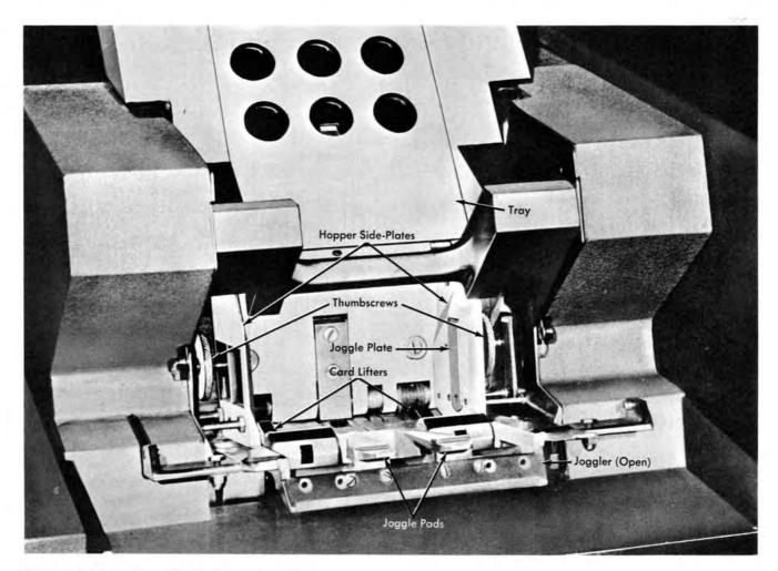
Figure 170. Interchangeable 51-Column Read Feed
