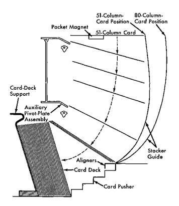
Figure 172. 51-Column Stacker Schematic
