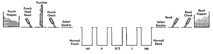
Figure 143. Punch Feed Read Schematic
