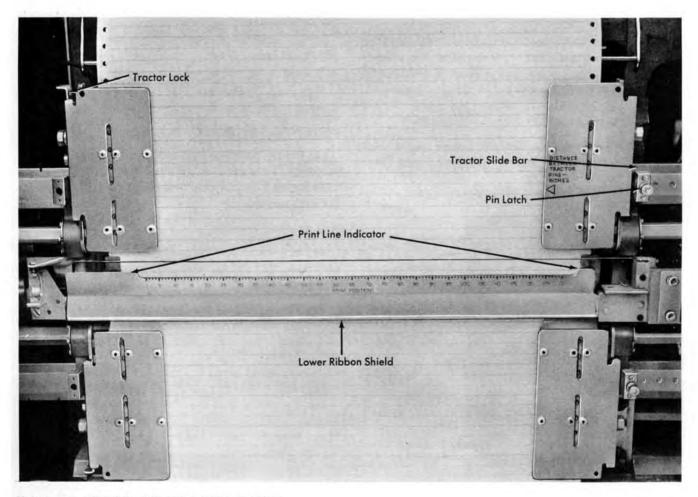
Figure 203. Print-Line Indicator and Ribbon Shield
