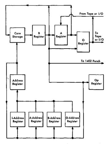
Figure 173. IBM 1401 Processing Overlap Data Flow
