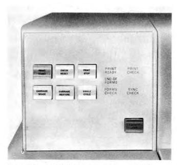
Figure 198. IBM 1403 Printer Operating Keys and Lights
