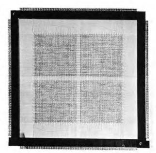
Figure 9. Magnetic Core Storage Unit
