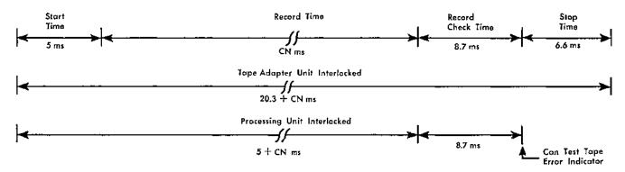
Figure 248. IBM 7330 Write Tape Timing
