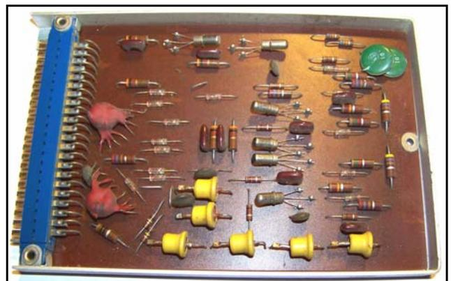
Shown above is an early DEC "Building Block" circuit board similar to the TX-0 and TX-2 technology. This is a flip-flop using Sprague transistors from 1959 (2N393s).
