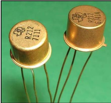
Transistor Size (1/4" Diameter X 1/4"H)
