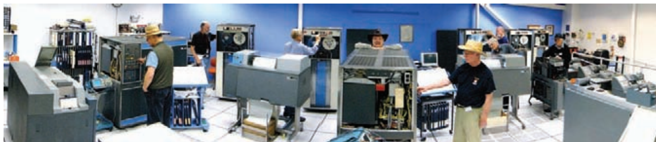
FIGURE 8: View of the 1401 restoration room at the CHM. The Connecticut 1401 is to the left of center, and the German 1401 is on the right. From left to right: Ron Williams, Don Luke, Joe Preston, Ed Thelen, George Ahearn, Frank King, Glenn Lea, and Bob Erickson (at an IBM 513 Reproducing Punch). An IBM 026 Printing Card Key punch and a 077 Collator are to the right. (Photo courtesy of Robert Garner.)
