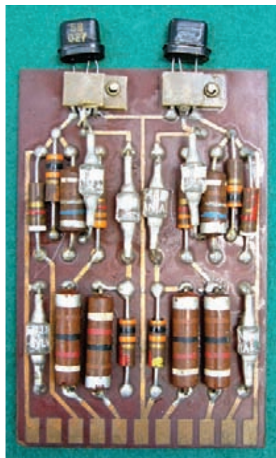
FIGURE 2: A printed-circuit logic card with germanium diodes and alloy-junction transistors from the 1955 experimental transistorized 604 calculator—basis of the IBM 608, world's first fully transistorized commercial calculator. (Photograph courtesy of Robert Garner.)
