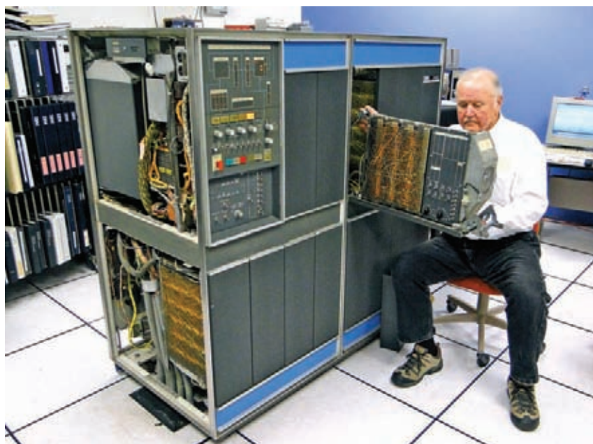
FIGURE 4: Restoration volunteer Ronald Williams and the 1401 processor "main frame" unit, which includes four SMS Cube frames with 24 gates of SMS cards (out of 32 total gate positions); the front panel with indicator lights, buttons, switches, and data paths; 4,000 positions of magnetic core memory; and hard-wired cable bundles to peripherals. The 1401 processor contains about 2,300 SMS cards with 10,600 alloy-junction transistors and 13,200 point-contact diodes. (Photo courtesy of Robert Garner.)
