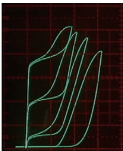
FIGURE 10: A current versus voltage trace of a defective germanium alloy-junction n-p-n transistor, illustrating a hysteresis curve likely caused by a surface inversion. The I-V curve shows collector-emitter voltage on the abscissa versus current on the ordinate at four different base currents. Such "loopy" I-V curves, measured with the collector voltage alternating from 2 Hz up to 1 MHz, appear to exhibit "memristor" behavior, first theoretically defined by Leon Chua in 1971 [17]. (Photo courtesy of Robert Garner.)
