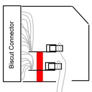
Two PCBs with rt angle 60-pin connectors.
