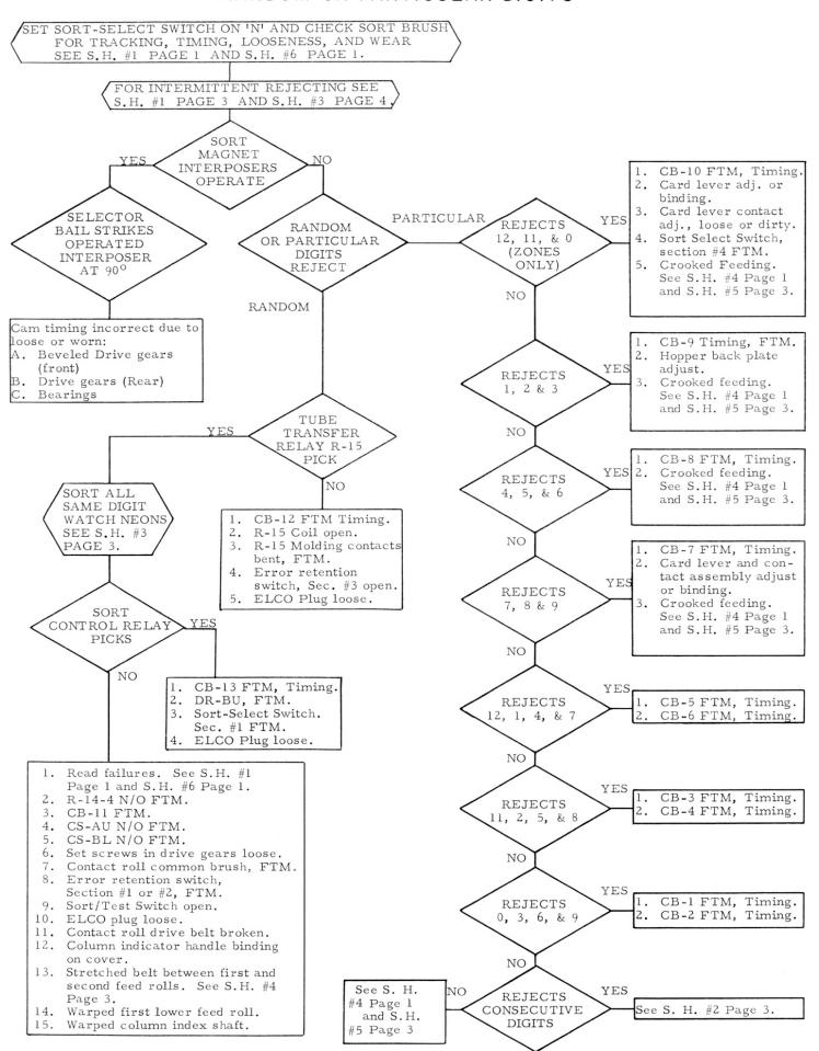
S.H. #1. Temporary Reject Detection Circuit
