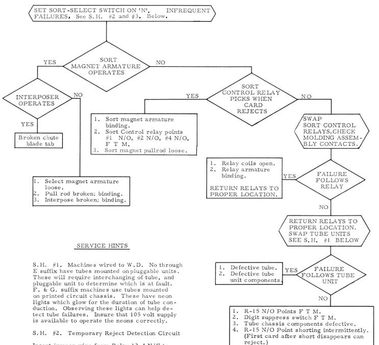
Insert jumper wire from Relay 12-4 N/C to Error Relay 16 Pl coil. Turn Edit Stop switch off. Run cards and sort on column containing numeric punches and no blanks or zones.
