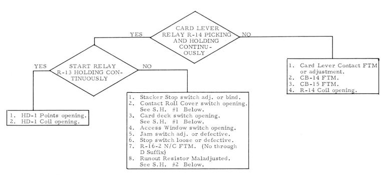
S.H. #1. Loose or maladjusted card deck or contact roll cover can cause stopping when cards are being joggled. Their respective switches may be properly adjusted, but the cover may cause them to open.
