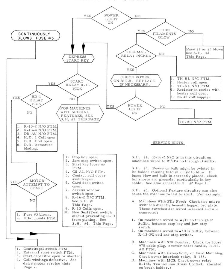
S.H. #4. Machines starting with K2 suffix incorporate a circuit change which prevents the machine from starting if the Sort/Test
