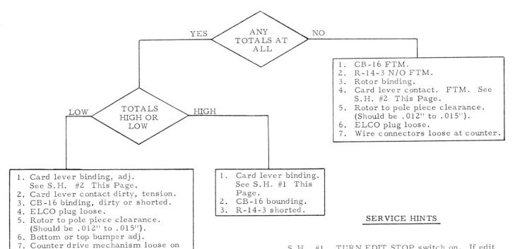
S.H. #1. TURN EDIT STOP switch on. If edit light appears on run out and counter total is high, check card lever.
