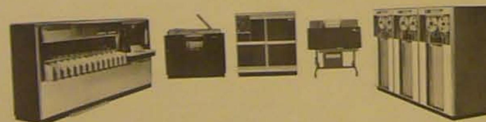
An IBM 1419 Magnetic Character Reader sorts checks as directed by the IBM 1401 Data Processing System which simultaneously prints multiple cash letter lists. Magnetic tape units shown are an optional part of the system.
