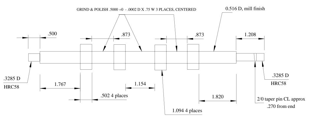
IBM 077 FEED SHAFT, AS MEASURED 1/4/2006
