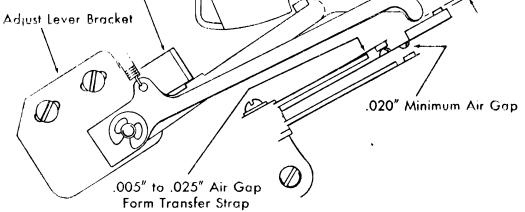
Figure 2. Program Cam Contact Bracket Adjustment
