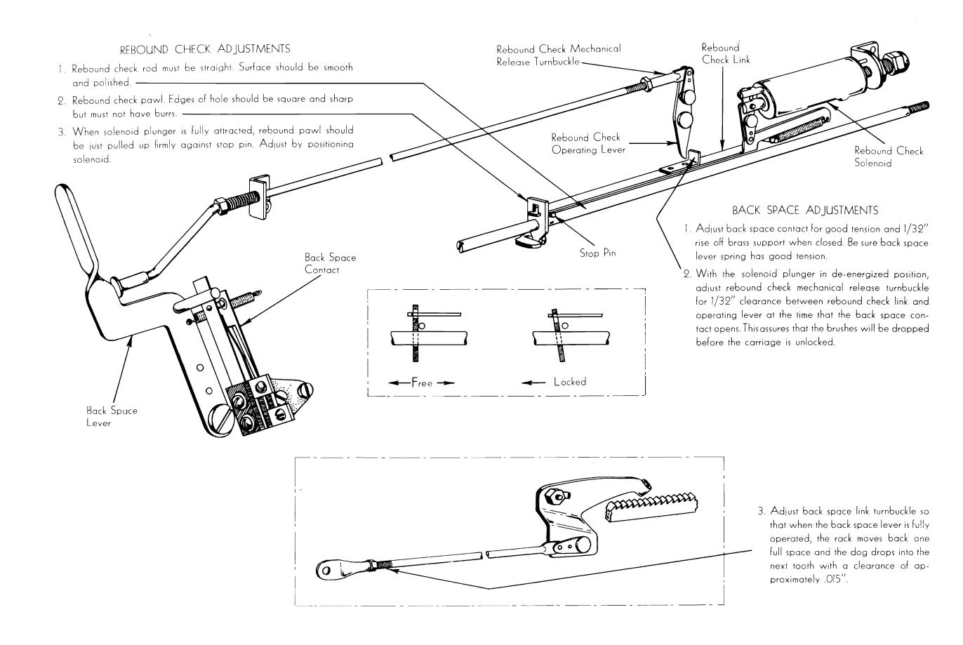
Remove the rebound check pawl. The edges of the hole should not be worn. They should be square and sharp but without burrs.
