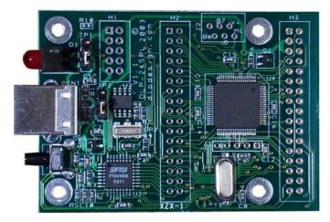
The DLP-245PL combines the same USB interface used in the DLP-USB245M module with a Microchip PIC microcontroller to form a rapid development tool. The 18LF8720 microcontroller is preprogrammed with basic functionality for accessing the port pins and can be reprogrammed with user hex code via a 5-pin header that is compatible with Microchip's MPLAB ICD2 device programmer/debugger (purchased separately).
