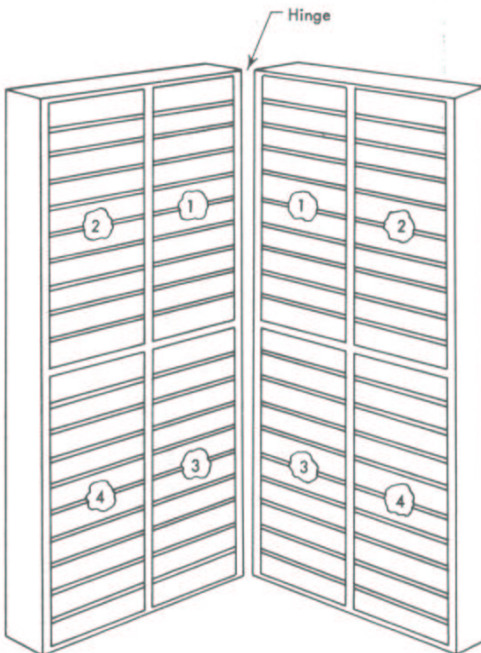
Figure 5-2. Module II Card Chassis (TAU I)
